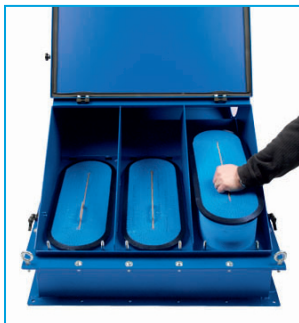
PowerCore filter pack can be lifted out & changed without tools at service time.
